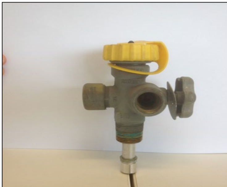
Figure 19. In-situ gas cylinder showing removable yellow cap
